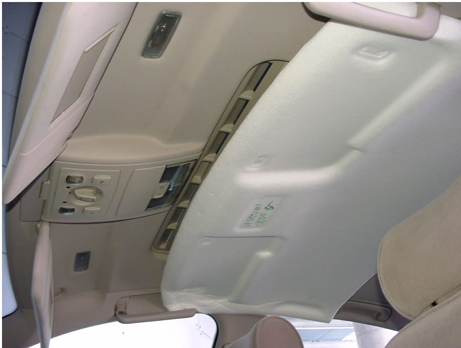
Figure 11: Roof liner made of compressed and formed non-woven with optimized acoustic absorption properties.
